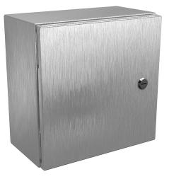
Wiegmann Ultimate series enclosure, NEMA 4/4X/12/13,  $12 \times 12 \times 6$  in (HxWxD), wall mount, 304 stainless steel, No. 3 intermediate polished finish, single-door, 1/4-turn semi-flush oil-tight latch.
