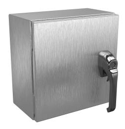
Wiegmann Ultimate series enclosure, NEMA 4X/12/13, 12 x 12 x 6in (HxWxD), wall mount, 304 stainless steel, No. 3 intermediate polished finish, single-door, 1-point 316L padlocking handle.
