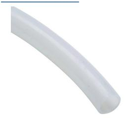
NITRA pneumatic tubing, nylon 12, natural, 3/8in outside diameter, 0.275in inside diameter, 100ft package.
