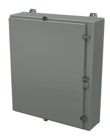
Stahlin N series enclosure, NEMA 1/3/3R/4X/12, 36 x 30 x 8in (HxWxD), wall mount, fiberglass reinforced polyester, gray, singledoor, (5) twist-lock latches, padlock hasp and staple.
