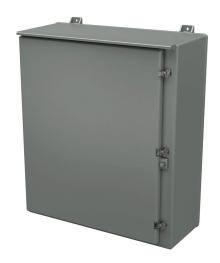
Stahlin N series enclosure, NEMA 1/3R, 36 x 30 x 12in (HxWxD), wall mount, fiberglass reinforced polyester, gray, single-door, (3) twist-lock latches, padlock hasp and staple.
