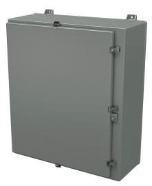
Stahlin N series enclosure, NEMA 1/3/3R/4X/12, 36 x 30 x 12in (HxWxD), wall mount, fiberglass reinforced polyester, gray, single-door, (5) twist-lock latches, padlock hasp and staple.
