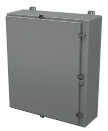
Stahlin N series enclosure, NEMA 1/3/3R/4X/12, 36 x 30 x 10in (HxWxD), wall mount, fiberglass reinforced polyester, gray, single-door, (5) twist-lock latches, padlock hasp and staple.
