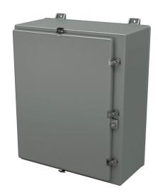
Stahlin N series enclosure, NEMA 1/3/3R/4X/12, 30 x 24 x 12in (HxWxD), wall mount, fiberglass reinforced polyester, gray, single-door, (5) twist-lock latches, padlock hasp and staple.
