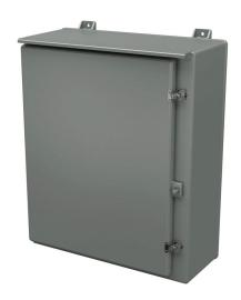
Stahlin N series enclosure, NEMA 1/3R, 30 x 24 x 10in (HxWxD), wall mount, fiberglass reinforced polyester, gray, single-door, (2) twist-lock latches, padlock hasp and staple.
