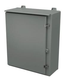
Stahlin N series enclosure, NEMA 1/3R, 30 x 24 x 10in (HxWxD), wall mount, fiberglass reinforced polyester, gray, single-door, (2) twist-lock latches, padlock hasp and staple.
