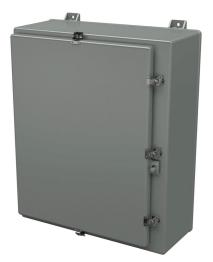
Stahlin N series enclosure, NEMA 1/3/3R/4X/12, 30 x 24 x 10in (HxWxD), wall mount, fiberglass reinforced polyester, gray, single-door, (5) twist-lock latches, padlock hasp and staple.
