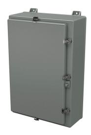
Stahlin N series enclosure, NEMA 1/3/3R/4X/12, 30 x 20 x 8in (HxWxD), wall mount, fiberglass reinforced polyester, gray, single-door, (5) twist-lock latches, padlock hasp and staple.
