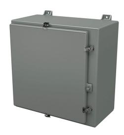
Stahlin N series enclosure, NEMA 1/3/3R/4X/12, 24 x 24 x 12in (HxWxD), wall mount, fiberglass reinforced polyester, gray, single-door, (4) twist-lock latches, padlock hasp and staple.
