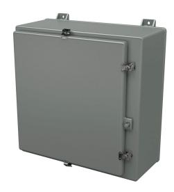
Stahlin N series enclosure, NEMA 1/3/3R/4X/12, 24 x 24 x 10in (HxWxD), wall mount, fiberglass reinforced polyester, gray, single-door, (4) twist-lock latches, padlock hasp and staple.
