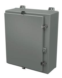
Stahlin N series enclosure, NEMA 1/3/3R/4X/12, 24 x 20 x 8in (HxWxD), wall mount, fiberglass reinforced polyester, gray, single-door, (4) twist-lock latches, padlock hasp and staple.
