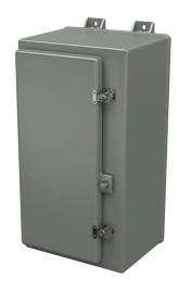
Stahlin N series enclosure, NEMA 1/3/3R/4X/12, 24 x 12 x 10in (HxWxD), wall mount, fiberglass reinforced polyester, gray, single-door, (2) twist-lock latches, padlock hasp and staple.
