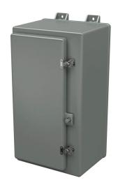
Stahlin N series enclosure, NEMA 1/3/3R/4X/12, 24 x 12 x 10in (HxWxD), wall mount, fiberglass reinforced polyester, gray, singledoor, (2) twist-lock latches, padlock hasp and staple.
