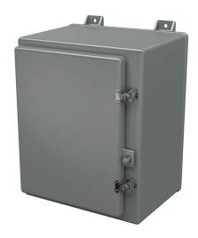
Stahlin N series enclosure, NEMA 1/3/3R/4X/12, 20 x 16 x 12in (HxWxD), wall mount, fiberglass reinforced polyester, gray, single-door, (2) twist-lock latches, padlock hasp and staple.
