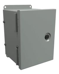
Hammond enclosure, 3-piece assembly, NEMA 1, 8 x 6 x 6in (HxWxD), wall mount, carbon steel, ANSI 61 gray, powder coat finish, single-door, 1/4-turn flush-mounted latch.
