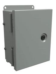
Hammond enclosure, 3-piece assembly, NEMA 1, 8 x 6 x 4in (HxWxD), wall mount, carbon steel, ANSI 61 gray, powder coat finish, single-door, 1/4-turn flush-mounted latch.
