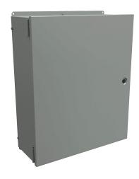
Hammond enclosure, 3-piece assembly, NEMA 1,  $24 \times 20 \times 8$ in (HxWxD), wall mount, carbon steel, ANSI 61 gray, powder coat finish, single-door, 1/4-turn flush-mounted latch.
