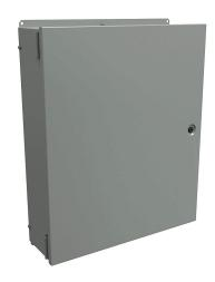
Hammond enclosure, 3-piece assembly, NEMA 1,  $24 \times 20 \times 6$ in (HxWxD), wall mount, carbon steel, ANSI 61 gray, powder coat finish, single-door, 1/4-turn flush-mounted latch.
