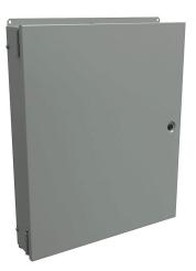
Hammond enclosure, 3-piece assembly, NEMA 1,  $24 \times 20 \times 4in$  (HxWxD), wall mount, carbon steel, ANSI 61 gray, powder coat finish, single-door, 1/4-turn flush-mounted latch.
