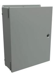
Hammond enclosure, 3-piece assembly, NEMA 1, 20 x 16 x 6in (HxWxD), wall mount, carbon steel, ANSI 61 gray, powder coat finish, single-door, 1/4-turn flush-mounted latch.
