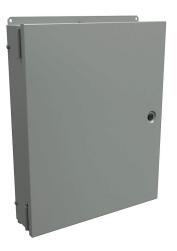
Hammond enclosure, 3-piece assembly, NEMA 1, 20 x 16 x 4in (HxWxD), wall mount, carbon steel, ANSI 61 gray, powder coat finish, single-door, 1/4-turn flush-mounted latch.
