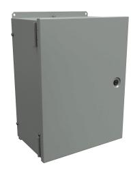
Hammond enclosure, 3-piece assembly, NEMA 1,  $16 \times 12 \times 8$ in (HxWxD), wall mount, carbon steel, ANSI 61 gray, powder coat finish, single-door, 1/4-turn flush-mounted latch.
