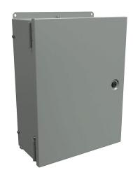
Hammond enclosure, 3-piece assembly, NEMA 1,  $16 \times 12 \times 6$ in (HxWxD), wall mount, carbon steel, ANSI 61 gray, powder coat finish, single-door, 1/4-turn flush-mounted latch.
