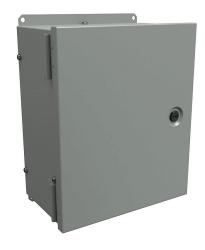
Hammond enclosure, 3-piece assembly, NEMA 1,  $12 \times 10 \times 6$ in (HxWxD), wall mount, carbon steel, ANSI 61 gray, powder coat finish, single-door, 1/4-turn flush-mounted latch.
