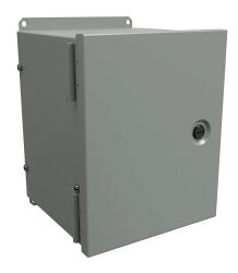
Hammond enclosure, 3-piece assembly, NEMA 1,  $10 \times 8 \times 8$  in (HxWxD), wall mount, carbon steel, ANSI 61 gray, powder coat finish, single-door, 1/4-turn flush-mounted latch.
