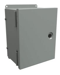
Hammond enclosure, 3-piece assembly, NEMA 1, 10 x 8 x 6in (HxWxD), wall mount, carbon steel, ANSI 61 gray, powder coat finish, single-door, 1/4-turn flush-mounted latch.
