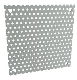
Hammond subpanel, perforated, carbon steel, ANSI 61 gray, powder coat finish. For use with 6x6 (HxW) N1J664 and C3R664HCR enclosures.
