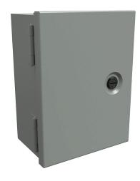
Hammond enclosure, NEMA 1,  $8 \times 6 \times 4$  in (HxWxD), wall mount, carbon steel, ANSI 61 gray, powder coat finish, single-door, 1/4-turn flush-mounted latch.
