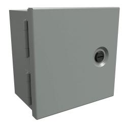
Hammond enclosure, NEMA 1, 6 x 6 x 4in (HxWxD), wall mount, carbon steel, ANSI 61 gray, powder coat finish, single-door, 1/4-turn flush-mounted latch.
