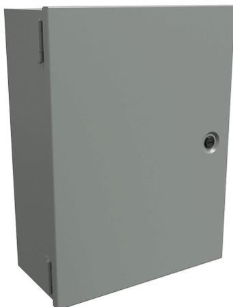
Hammond enclosure, NEMA 1, 16 x 12 x 6in (HxWxD), wall mount, carbon steel, ANSI 61 gray, powder coat finish, single-door, 1/4-turn flush-mounted latch.
