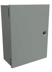
Hammond enclosure, NEMA 1,  $16 \times 12 \times 6$  in (HxWxD), wall mount, carbon steel, ANSI 61 gray, powder coat finish, single-door, 1/4-turn flush-mounted latch.
