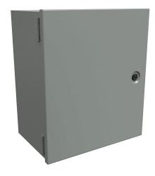
Hammond enclosure, NEMA 1, 14 x 12 x 8in (HxWxD), wall mount, carbon steel, ANSI 61 gray, powder coat finish, single-door, 1/4-turn flush-mounted latch.
