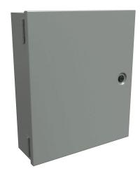
Hammond enclosure, NEMA 1, 14 x 12 x 4in (HxWxD), wall mount, carbon steel, ANSI 61 gray, powder coat finish, single-door, 1/4-turn flush-mounted latch.
