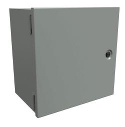
Hammond enclosure, NEMA 1, 12 x 12 x 8in (HxWxD), wall mount, carbon steel, ANSI 61 gray, powder coat finish, single-door, 1/4-turn flush-mounted latch.
