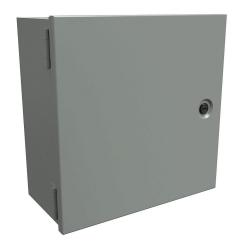
Hammond enclosure, NEMA 1, 12 x 12 x 6in (HxWxD), wall mount, carbon steel, ANSI 61 gray, powder coat finish, single-door, 1/4-turn flush-mounted latch.
