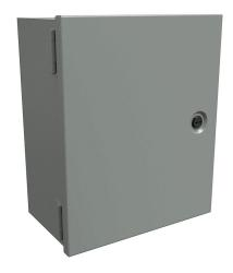
Hammond enclosure, NEMA 1, 12 x 10 x 6in (HxWxD), wall mount, carbon steel, ANSI 61 gray, powder coat finish, single-door, 1/4-turn flush-mounted latch.
