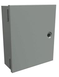
Hammond enclosure, NEMA 1, 12 x 10 x 4in (HxWxD), wall mount, carbon steel, ANSI 61 gray, powder coat finish, single-door, 1/4-turn flush-mounted latch.
