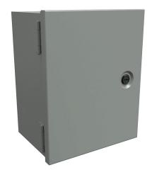
Hammond enclosure, NEMA 1, 10 x 8 x 6in (HxWxD), wall mount, carbon steel, ANSI 61 gray, powder coat finish, single-door, 1/4-turn flush-mounted latch.
