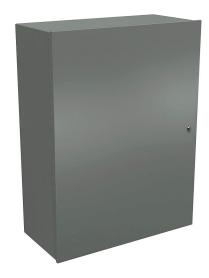
Wiegmann enclosure, NEMA 1, 48 x 36 x 17in (HxWxD), wall mount, carbon steel, ANSI 61 gray, powder coat finish, single-door, 1/4-turn flush-mounted latch.
