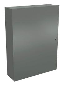
Wiegmann enclosure, NEMA 1, 48 x 36 x 11in (HxWxD), wall mount, carbon steel, ANSI 61 gray, powder coat finish, single-door, 1/4-turn flush-mounted latch.
