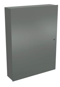
Wiegmann enclosure, NEMA 1, 48 x 36 x 9in (HxWxD), wall mount, carbon steel, ANSI 61 gray, powder coat finish, single-door, 1/4-turn flush-mounted latch.
