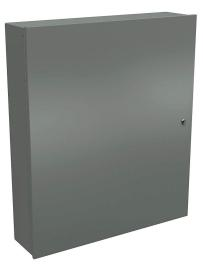
Wiegmann enclosure, NEMA 1, 42 x 36 x 9in (HxWxD), wall mount, carbon steel, ANSI 61 gray, powder coat finish, single-door, 1/4-turn flush-mounted latch.
