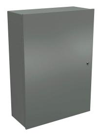
Wiegmann enclosure, NEMA 1, 42 x 30 x 13in (HxWxD), wall mount, carbon steel, ANSI 61 gray, powder coat finish, single-door, 1/4-turn flush-mounted latch.
