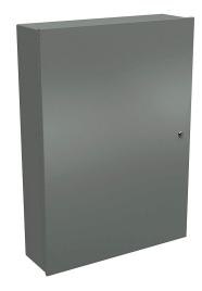
Wiegmann enclosure, NEMA 1, 42 x 30 x 9in (HxWxD), wall mount, carbon steel, ANSI 61 gray, powder coat finish, single-door, 1/4-turn flush-mounted latch.
