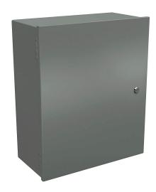
Wiegmann enclosure, NEMA 1, 24 x 20 x 10in (HxWxD), wall mount, carbon steel, ANSI 61 gray, powder coat finish, single-door, 1/4-turn flush-mounted latch.
