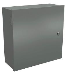
Wiegmann enclosure, NEMA 1, 20 x 20 x 8in (HxWxD), wall mount, carbon steel, ANSI 61 gray, powder coat finish, single-door, 1/4-turn flush-mounted latch.
