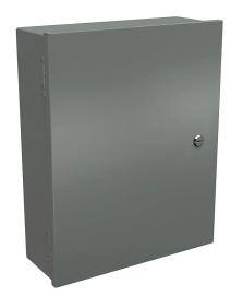
Wiegmann enclosure, NEMA 1, 20 x 16 x 6in (HxWxD), wall mount, carbon steel, ANSI 61 gray, powder coat finish, single-door, 1/4-turn flush-mounted latch.
