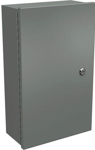
Wiegmann enclosure, NEMA 1, 20 x 12 x 6in (HxWxD), wall mount, carbon steel, ANSI 61 gray, powder coat finish, single-door, 1/4-turn flush-mounted latch.
