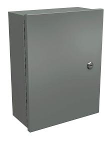
Wiegmann enclosure, NEMA 1, 16 x 12 x 6in (HxWxD), wall mount, carbon steel, ANSI 61 gray, powder coat finish, single-door, 1/4-turn flush-mounted latch.
